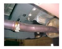
TO REMOVE YOUR STOCK EXHAUST, REMOVE IT FROM THE CLAMP LOCATED JUST IN FRONT OF THE MUFFLER AND REMOVE HANGERS FROM RUBBER GROMMETS BY PULLING EXHAUST TOWARDS THE REAR OF THE VEHICLE, USE WD-40 TO AID IN REMOVAL, LEAVE GROMMETS IN PLACE.
